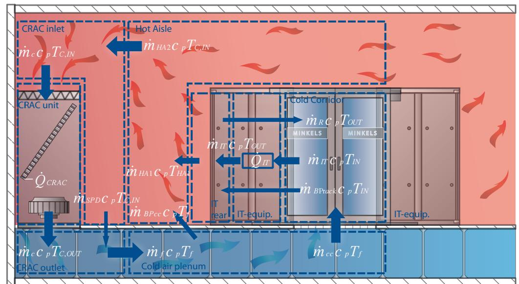
Based on the boundary conditions illustrated in figure A1 the following schematic representation is used to derive the formulas:
