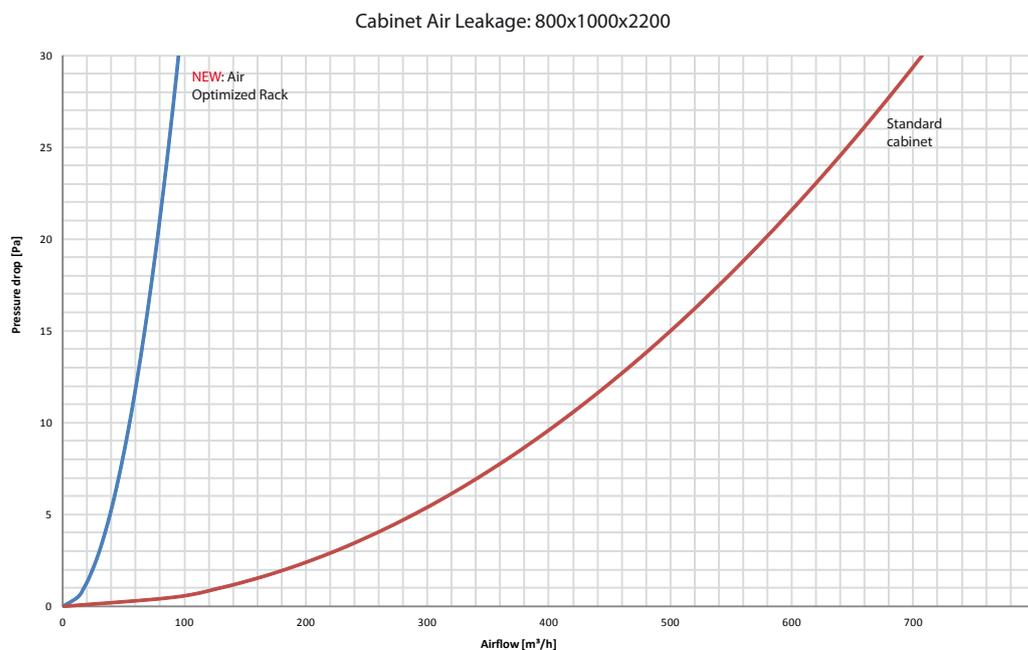
The new improved racks shows a considerable improvement. When it is assumed that inside a cold corridor there exists a differential pressure of 5 Pa towards the hot corridor the improved rack reduces the air losses by 86% per rack. This is truly remarkable.
